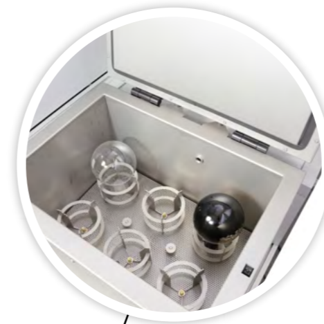
Washing chamber in the module bitumen washing machine
