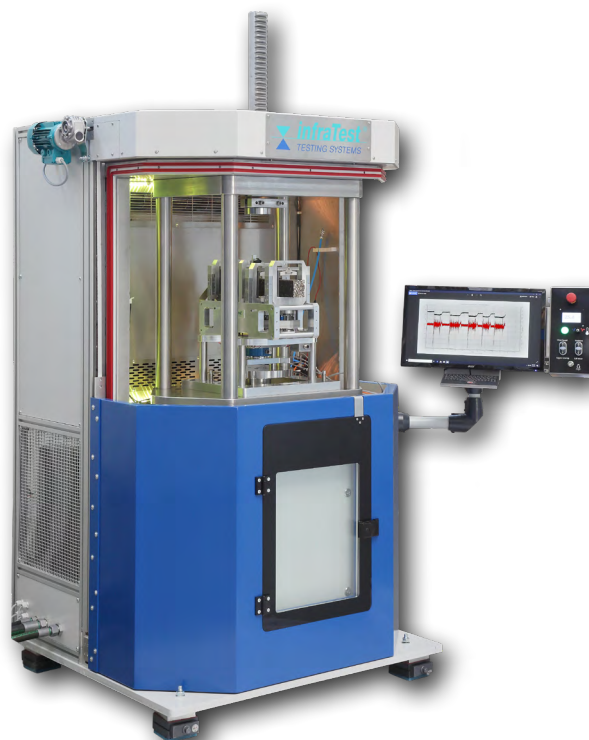
Drive cylinder from above is absolutely necessary for layer bond tests and TRAVIS
