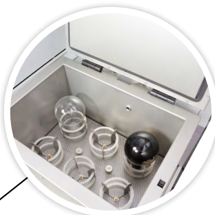
Washroom in the parts cleaning module
